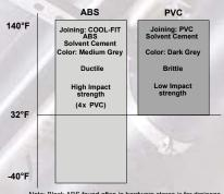
Note: Black ABS found often in hardware stores is for drainage and not designed for pressure systems or cold temperatures
