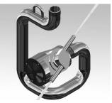
Lechler offers a special mounting attachment which allows the M20 BRDRV version to double the spray effectiveness on the end bulkheads of long, horizontal tanks or tankers. The mounting part number is 099.164.17.00.
