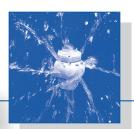
While PTFE can withstand high temperatures, its dimensional stability limits its range as a tank cleaning device. Lechler's new design incorporates Hastelloy® rings to control the expansion of the material so it can continue to operate reliably in hotter environments than normally possible. The range is actually extended, since it can perform equally well under normal conditions. The spray characteristics are the same as the standard units.
